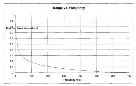
Assuming a transmit power reference and a static distance, different frequencies will result in different path losses from which the received signal levels can be derived. For convenience of use, ranges have been defined. The main challenge is to select the ranges so as to contain bands allocated for the same purpose. By doing so, there will be only minimal disparity between licensees using different frequency
